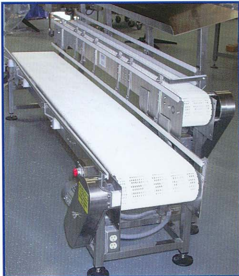
Pack Off Conveyor Station
